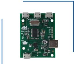
The oSynC-3U OTG's Micro USB ports allow you to connect up to three peripherals, such as a scanner, printer and card reader. It is ideal for running mobile-based staff time clocks, warehouse management systems or retail kiosks.
